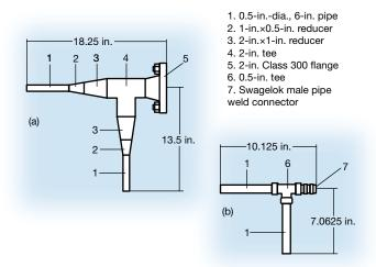
▲ Figure 3. (a) Large flanged thermowells introduce residence time issues in pilot plants, which have smaller piping. (b) Swaging the thermocouple directly into the process line is a more appropriate and scale-specific method of temperature measurement that lowers residence time because of the smaller volume.
