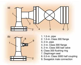
▲ Figure 2. (a) When piping specifications for a commercial plant are applied to measure differential pressure across a pilot-scale reactor, the incompatible piping creates a large dead volume that affects product quality and the ability to control temperature. (b) Replacing the entire assembly with a smaller-scale solution minimizes the dead volume and helps to control the reactor temperature profile.
